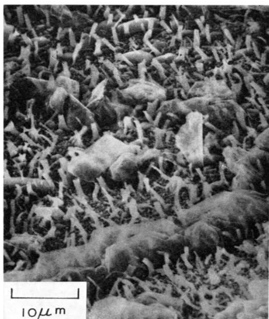
Fig. 1. Effect of inadequate cleaning on the formation of whiskers.
